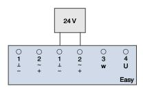
The supply voltage and the remote room temperature controller must be connected as shown.
